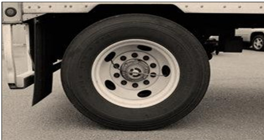
Figure 10.3: Automatic Tire Inflation System Installed on Truck
