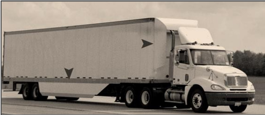
Figure 10.2: Covering the Gap between Cabin and Trailer
